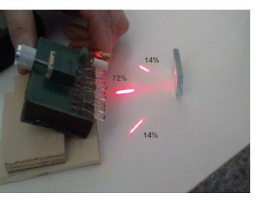
In this second image you can see that adding a mirror increases the brightness by almost three times.
