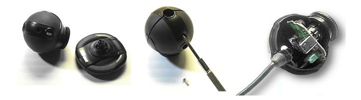
Separate the chamber from the base and unscrew the small screw that holds the two halves of the shell together. Separate the two halves of the shell by pulling hard, without fear, at the end the shell will split and you can extract the printed circuit board.
