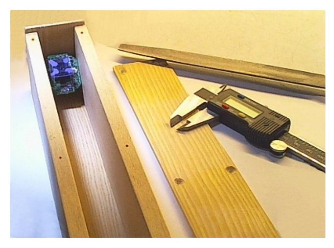
With wood and small screws, you can build lightweight containers that are easy to open on each side and easy toedit for testing.
