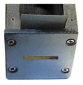
When screwing the cover on, leave enough space for the diaphragm.
