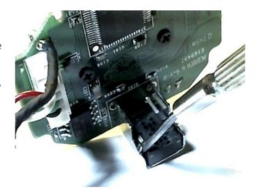
If the button terminals are still attached to the PCB, cut them off at the base using wire cutters or small scissors.
