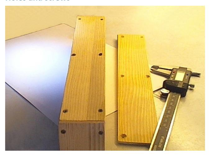
All holes should be made on the 4mm pieces. On the two long pieces, make six holes, three on each side. On the two terminals, make four holes. The holes should be made with a 2.5mm bit and should all be 5mm from the edge. Finally, the holes should be countersunk with a large drill bit (about 6mm).
